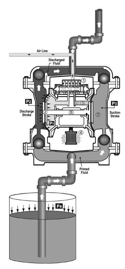
VERSA-MATIC<sup>®</sup> u2nmsm-rev0817 Air-Operated Double Diaphragm (AODD) pumps are powered by compressed air or nitrogen.
